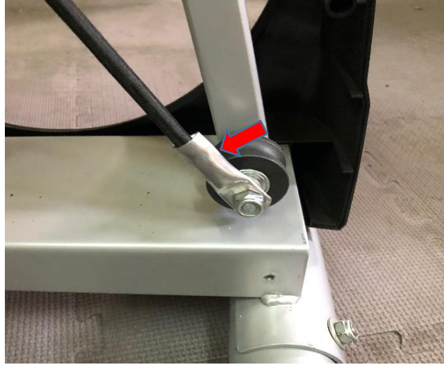
Step 2: Lock the nuts and strap's angle like this.
